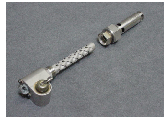
Fuel metering, vaporization and mixing assembly
