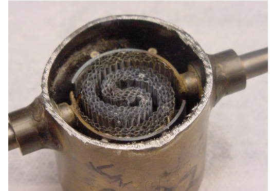
Electrically heated catalyst and start-up strategy development
