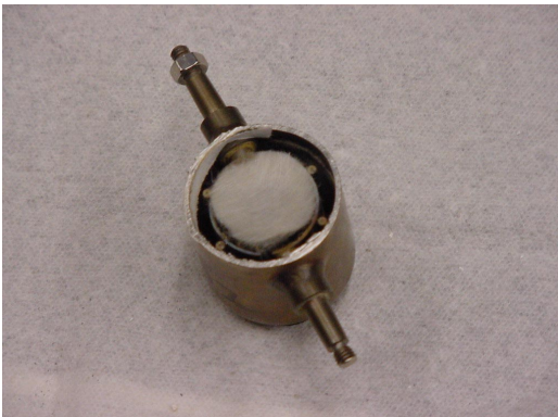
Reformer catalyst inlet flame arrestor / radiation shield
