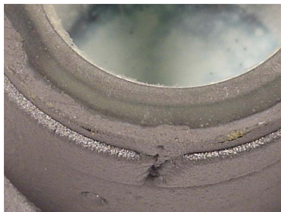
Figure 3.2-35 Photographs of coated Textron substrate (test coating #4) as viewed from the bottom of the graphite cylinder pedestal. Notice the white powdery substance deposited on the inside walls of the cylinder. This is attributed to out-gassing of the Textron SiC/Si 3 N 4 composite material.
