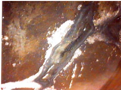
Figure 3.3-79 This crack near the dome end of the tube is wetted with aluminum throughout the wall thickness.
