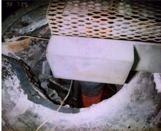
Figure 3.3-24 Cold Start up – Ingots partially melted
