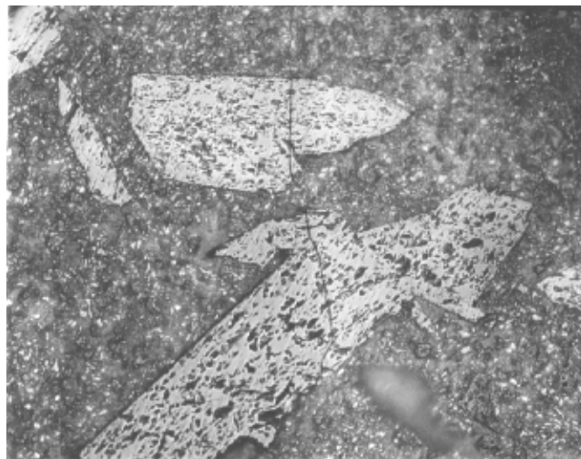
Figure 3.4.8 Matrix cracking was observed in 2-D composite after thermal shock test at \Delta T of 1000°C.
