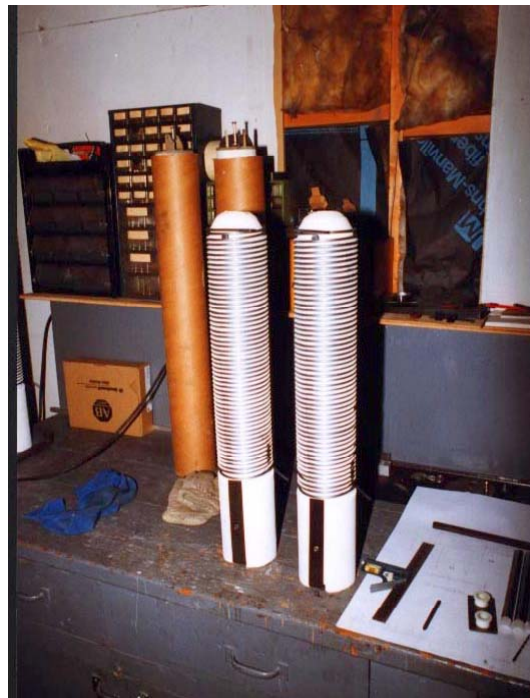
Figure 3.3-25 The electric heating element being used in immersion tube #6 at GM Advanced Development Center in Saginaw, MI
