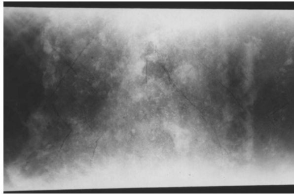
Figure 3.3-57 Radiograph Tube #8 Cracks - 240°
