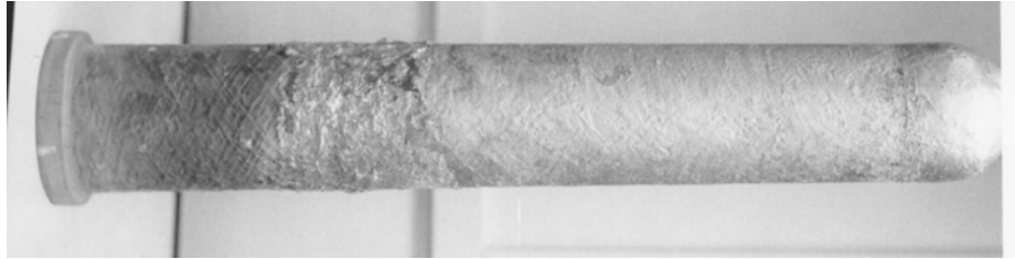
Figure 3.3-54 Tube No. 8 – 1750 Hours of Service – 49 Thermal Cycles
