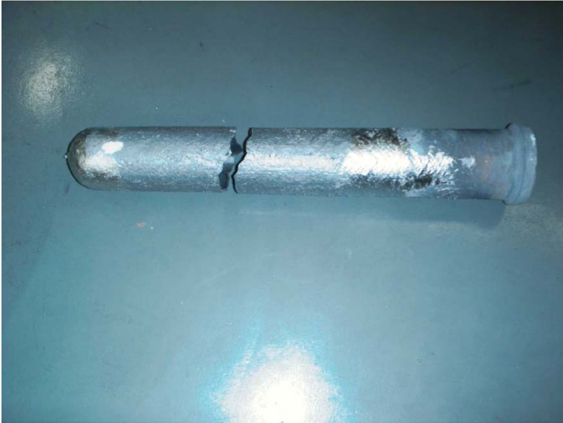
Figure 3.3-27 Immersion Tube No. 6 Fracture
