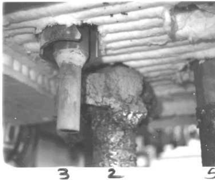
Figure 3.3-4 Shows complete fracture of burner 3 at the meltline. A significant corundum bloom existed on the missing half of the tube.
