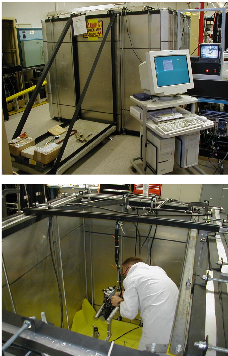
Figure 4-4. Photograph of the completed shield assembly used for the ^{225}\text{Ac} experiment. In the upper photograph, the braced structure with warning sign attached is the door to the experimental chamber. Also visible in the photograph are the computer workstation and NIM and CAMAC electronic assemblies used to control the experiment. In the lower photograph, a worker is shown configuring the detector assembly for the ^{225}\text{Ac} experiment. The cast iron angle bracing that supports the neutron shield is also clearly visible in this photograph.
