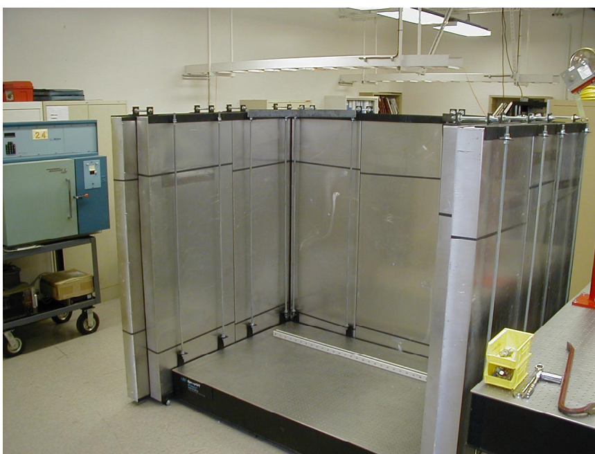
Figure 4-3. Photographs of the initial assembly of the shield arrangement used for the ^{225}\text{Ac} experiment. The upper photograph shows one panel of the borated polyethylene shield (in its aluminum case) being placed in its position adjacent to the optical table. The lower photograph shows three panels of the borated shield around the optical table, as well as the cast-iron framework to support the shields.
