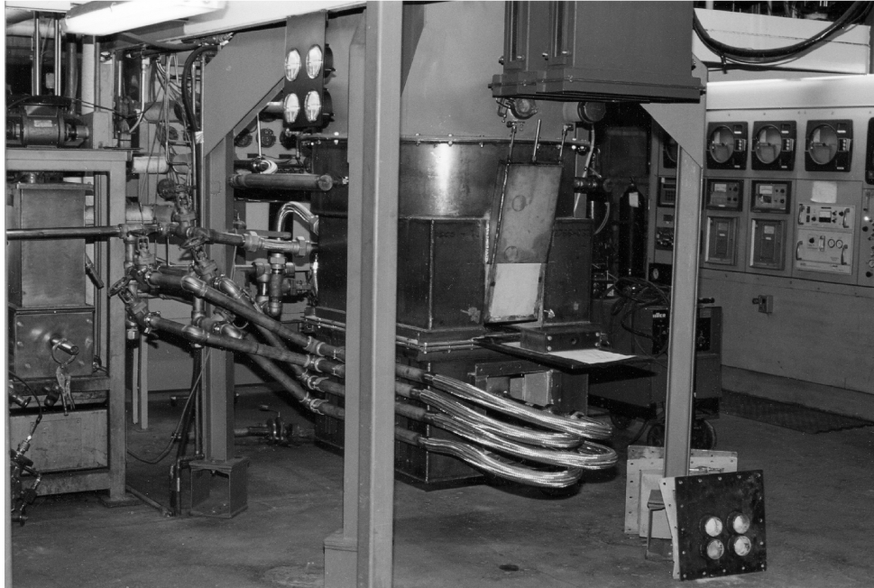
Figure 5. Photograph of grate-fired system components installed on CTF.
