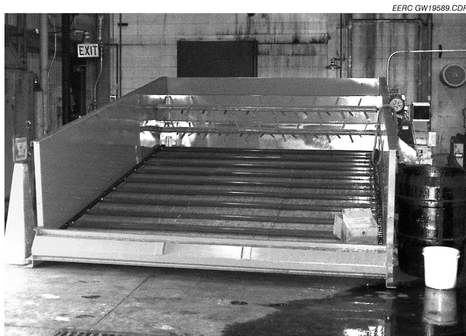
Figure 7. Photograph of table feeder.
