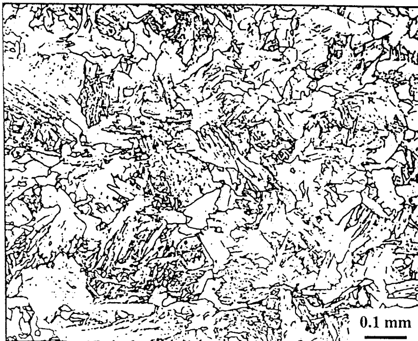
Figure 2-6: Commercial strip cast material: transverse section, acicular ferrite microstructure, 2% Nital etch, 100x
