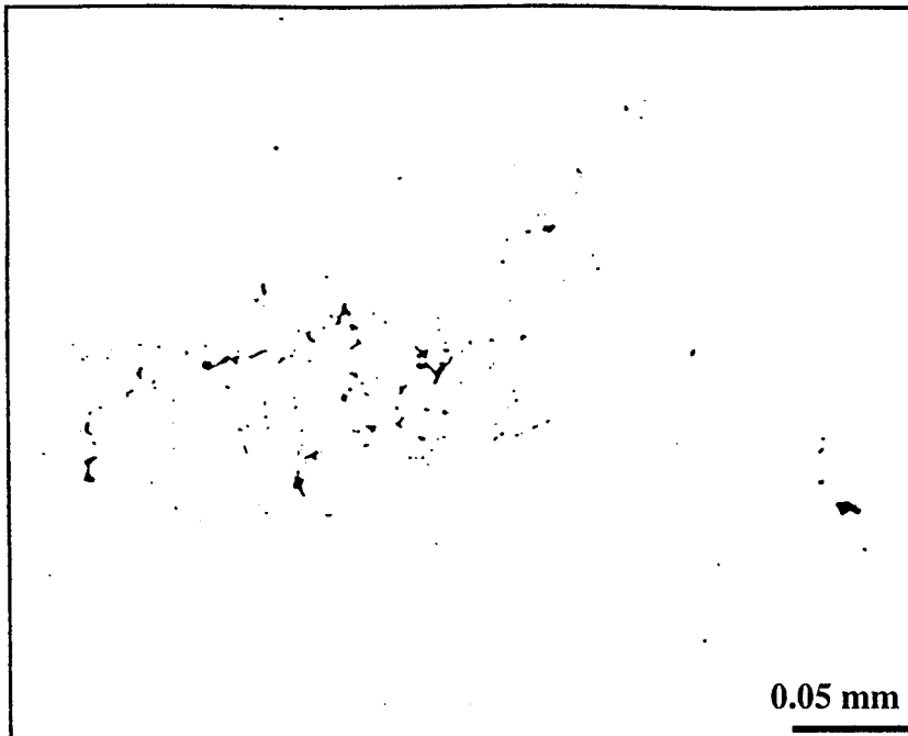
Figure 2-19: British Steel Low Carbon Steel Strip Cast Material - longitudinal section; Si-killed- Inclusions and porosity throughout the material, Unetched 200x
