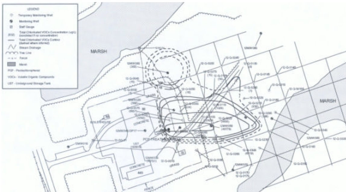
Figure 2. Contour map showing the total chlorinated solvent concentrations in the upper surficial aquifer at the SWMU-12 site. The outer dashed contour line is zero concentration and the inner contour line is 30,000 micrograms per liter.
