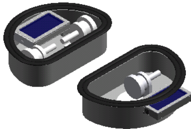
Figure 7. Detectors Integrated into the IVOD's Suction Chambers.
