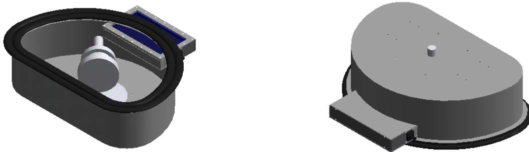
Figure 8. SP-Series Detectors Front Chamber Location.
