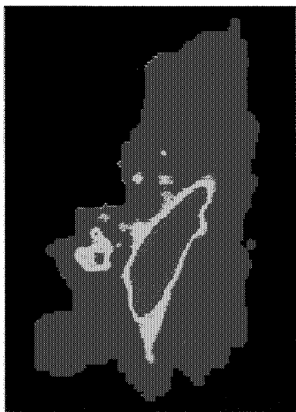
Figure 40: Time-lapse difference mapped on the 4500-ft horizon, showing the change in amplitudes of the stacked seismic data between Phase I and Phase II, the two OBC time-lapse surveys. The 4500-ft reservoir and the Little Neighbor reservoir both show significant changes indicated by the blue and green colors, although only the larger 4500-ft reservoir is under production. (Image provided by W. Haggard, C. Vuillermoz, S. Spitz, and P. Granger of CGG, presented to the ERCH consortium in August, 2000.)
