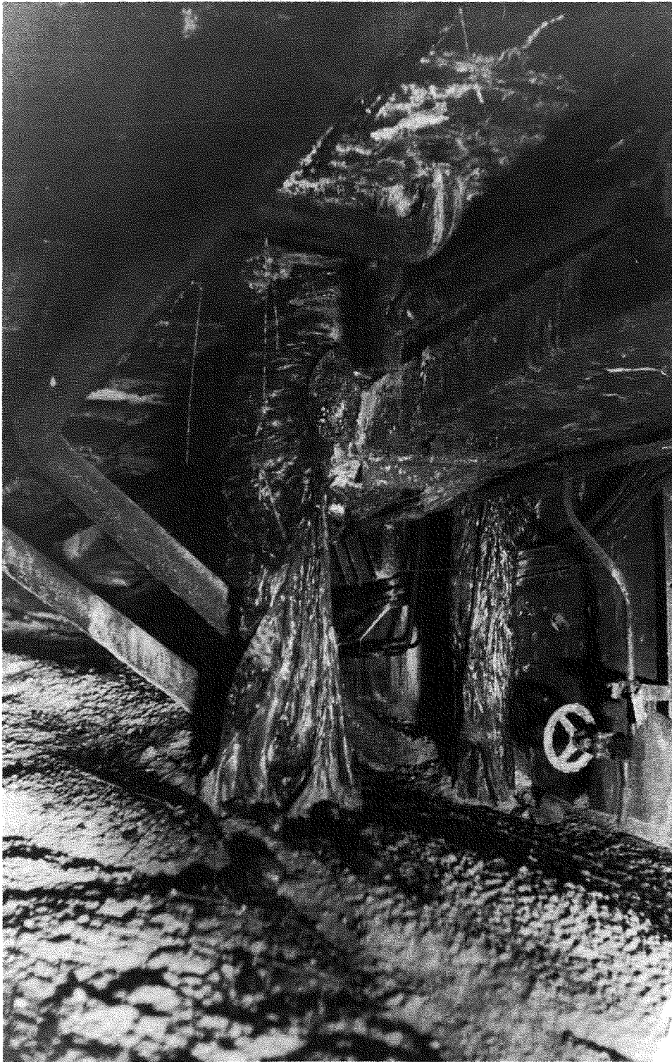
Fig. 12 Photograph of a nuclear fuel stalactite located near the southern end of Corridor 217/2. (Photograph courtesy of Aleksandr Aleksandrovich Borovoi of the Inter-Branch Scientific and Technical Center "Shelter.")
