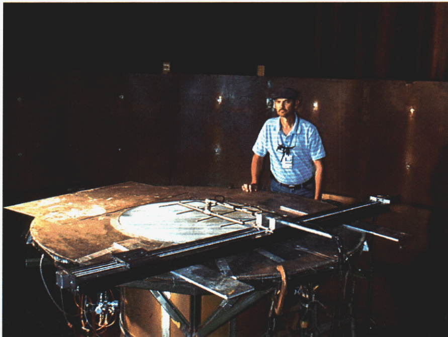
Figure 27. Scanning the plume source with 4 TSI hot-wire probes on 6-ft X-Y table.
