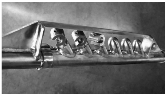
Electrode detail showing new gasket design: C-ring channel and bullet electrode channel
