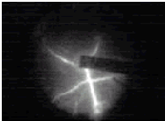
Figure 2. Luminous reaction in cracks of PBX 9501 during mechanically coupled cookoff experiment from Dickson et al.(5)
