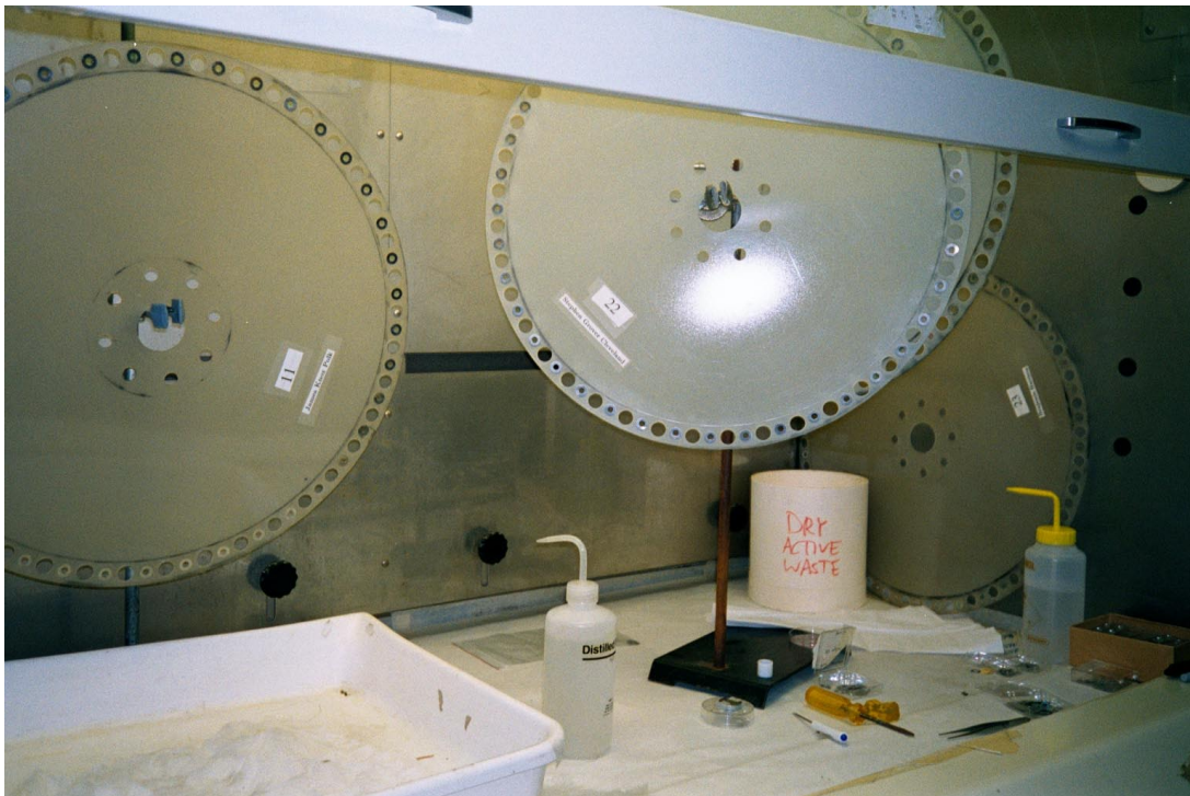
Photograph D.7: The MG wheel washing and inspection during the ^{266}\text{Bh} run.
