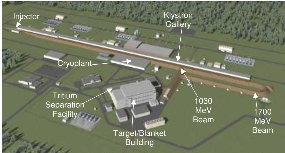
Figure 4. Reference Design APT Layout
