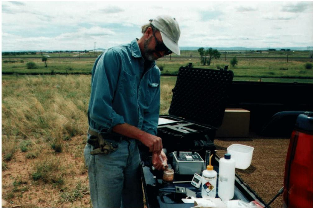
**Figure 2. Diesel Dog Soil Test Kit Field Use**
