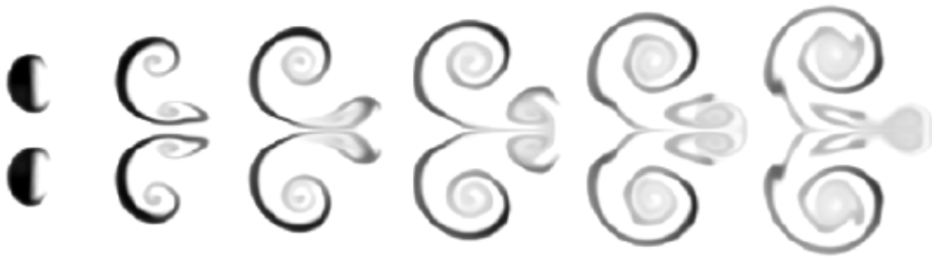
Figure 6. Simulated density field of two spanwise-interacting cylinders for S = 2.0D . Data presented at t = 50, 190, 330, 470, 610 , and 750 \mu\text{s} after shock impact.
