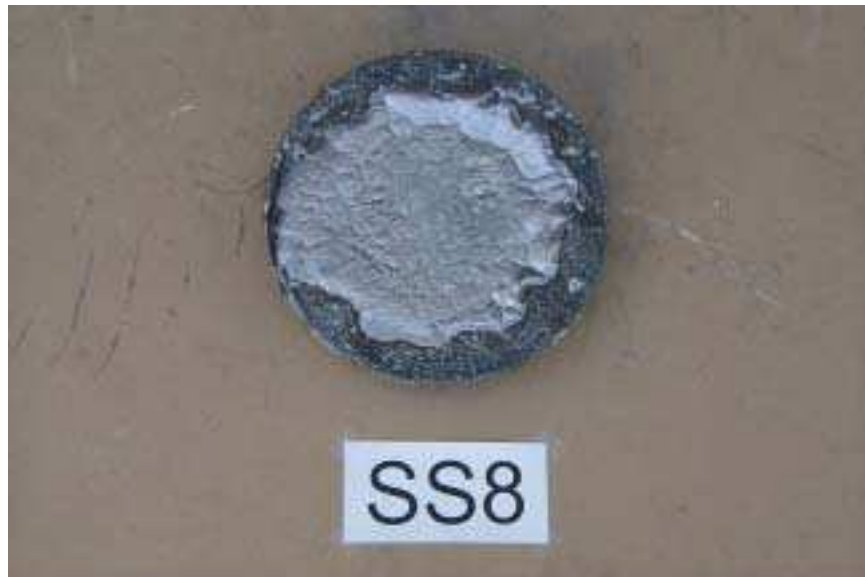
Figure 1. Front side of SS ingot after SS Melt Test #8. The graphite susceptor is seen between the two SS ingots.
