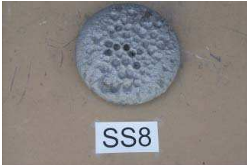
Figure 2. Reverse side of SS ingot after SS Melt Test #8.
