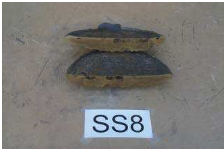
Figure 3. Cross section of SS ingot after SS Melt Test #8.
