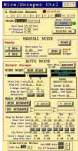
Figure 2: Operator Control Screen for Scans and Scrapes
