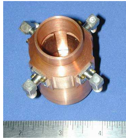
Figure 1: Prototype drift tube BPM. Vacuum connectors from Kaman will be used on the final BPMs.
