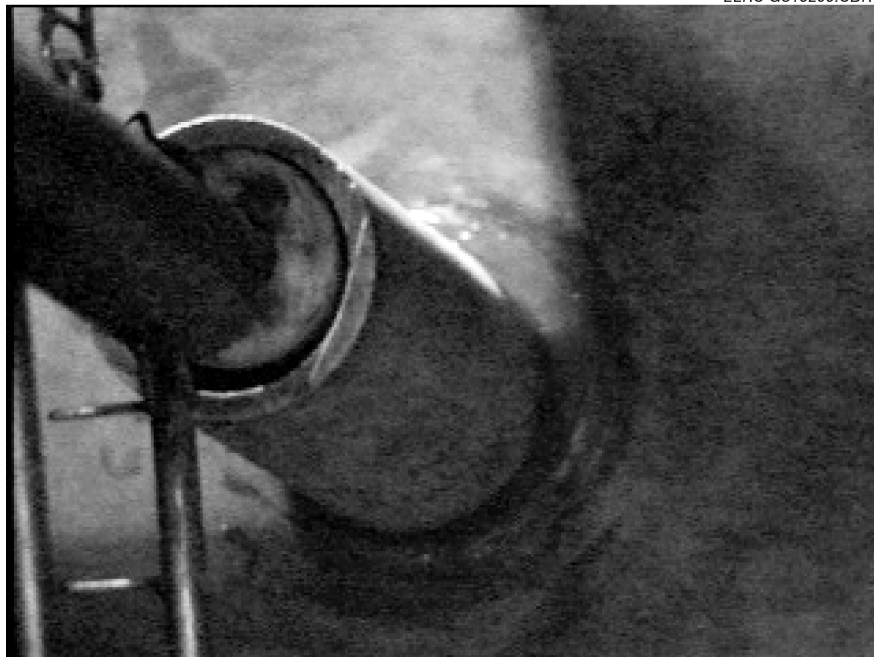
Figure 4.1-22. The ceramic sheath covering the PTFE high-voltage power coupling.
