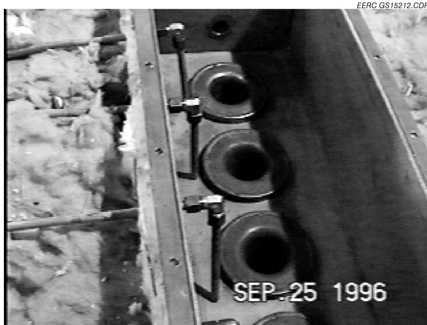
Figure 4.1-25. Pulse-jet bag-cleaning assembly modified to pulse each bag one at a time.
