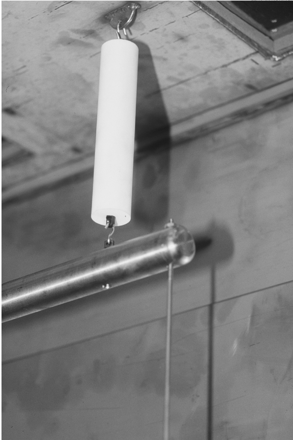
Figure 4.1-12. One of the machinable ceramic insulators supporting the ESP grid.
