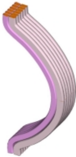
Figure 2. ARIES-AT outboard first wall and blanket.
