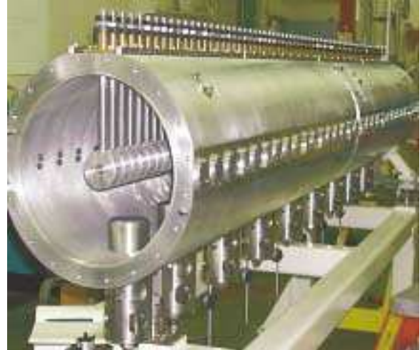
Figure 1. Full-scale aluminum model of DTL tank 1.
