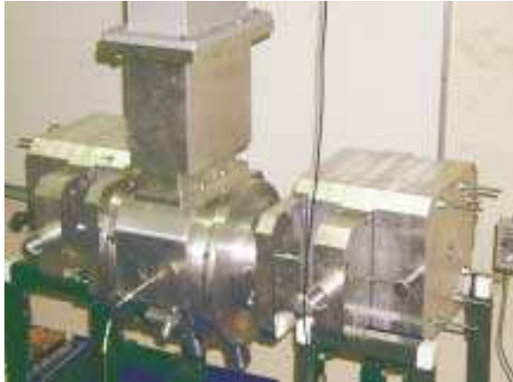
Figure 4. CCL aluminum model of bridge coupler between two 4-cavity segments and connected to the waveguide.
