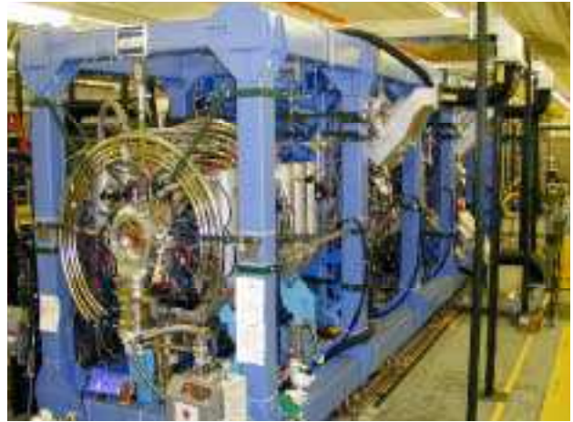
Figure 3: A photograph of the RFQ mounted in the support/alignment frame, looking along the beam direction. The accelerating structure is buried within the array of water-cooling manifolds, vacuum manifolds, and RF waveguide.
