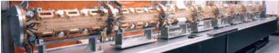
Figure 1: Eight-meter-long RFQ in the tuning laboratory. The adjustable slug tuners can be seen in this picture.
