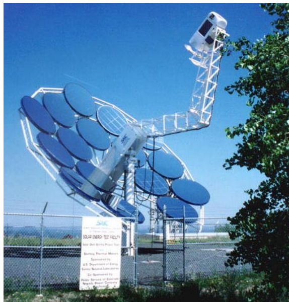
Figure 1. Phase 1 SAIC/STM Prototype Dish/Stirling System
