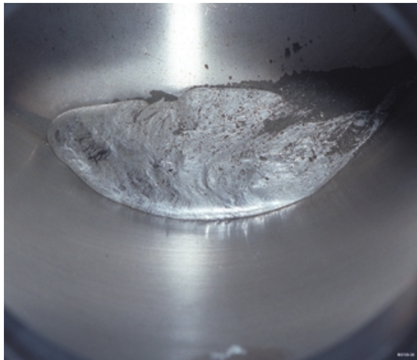
4. Liquid Indalloy 51 in reactor with powdered corrosion product after the test.
