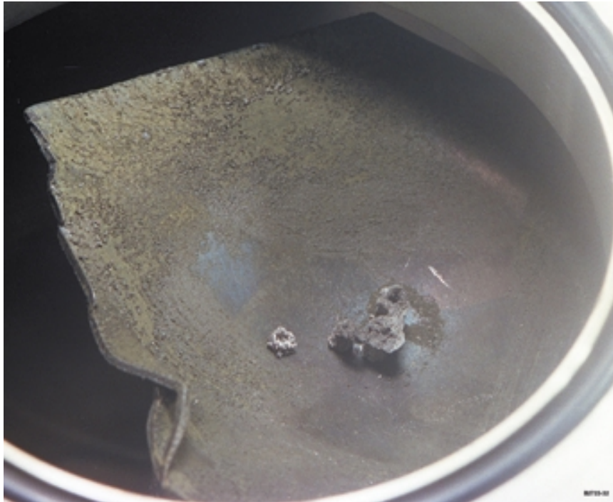
3. Solid residual test material in the plutonium cup and adjacent plutonium surface after the test.
