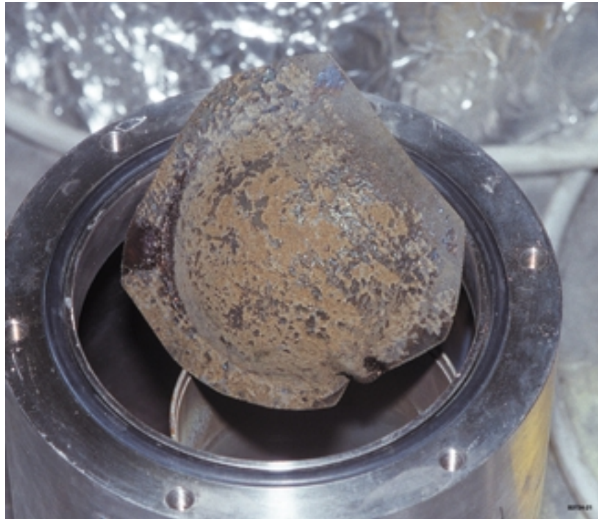
5. Convex surface of the plutonium specimen after the test.
