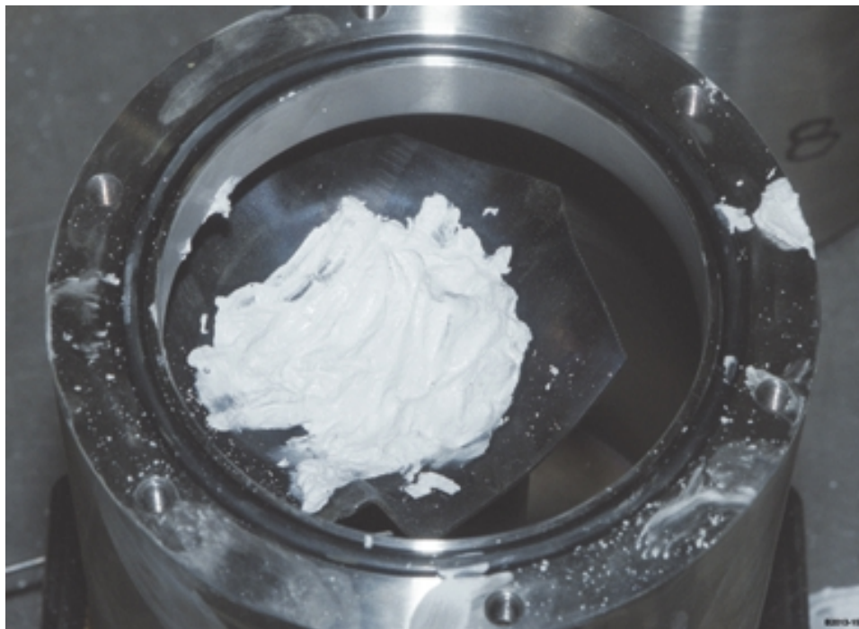
2. MgO + H 2 O + ethylene glycol slurry in the plutonium cup before the test.
