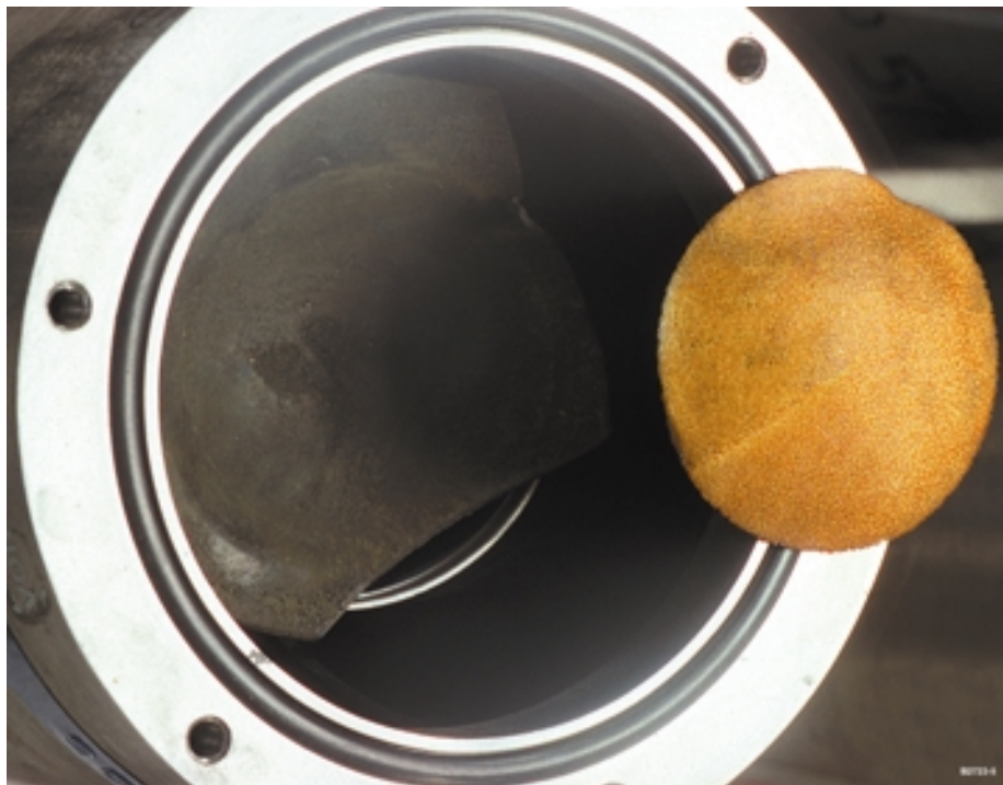
4. Contact surface of the residual test material and surrounding plutonium surface after the test.
