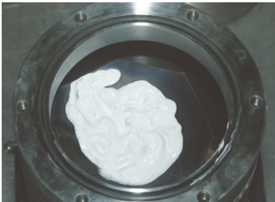
2. MgO + H 2 O slurry in the plutonium cup before the test.
