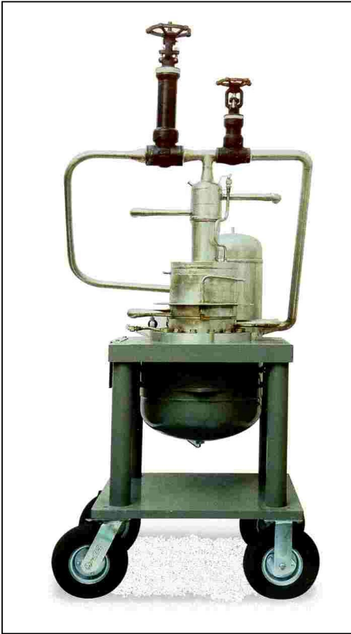
Figure 5. An early prototype linear compressor driven OPTR
