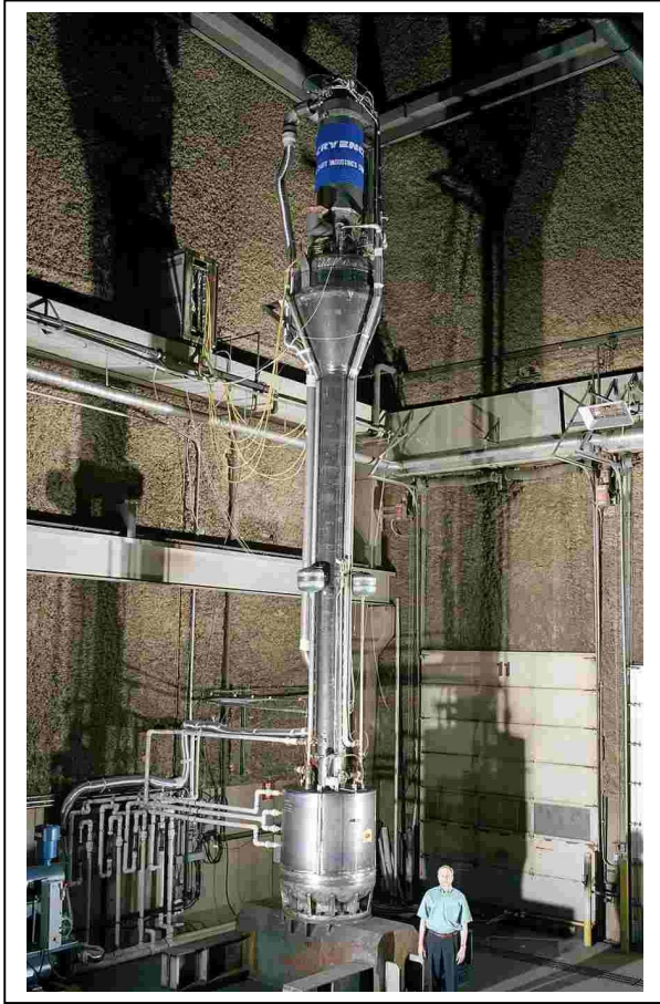
Figure 2. The 500 gpd TASHE-OPTR. The natural gas burner is at the very top. The TASHE is the large bulge below the burner and the OPTRs (not visible) are inside the vacuum jacket near the bottom.
