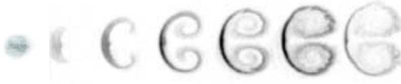
Fig. 1. Initial conditions ( t = 0 ) and dynamic images ( t = 50, 190, 330, 470, 610, 750 \mu\text{s} after shock impact) of shock-accelerated gas cylinder
