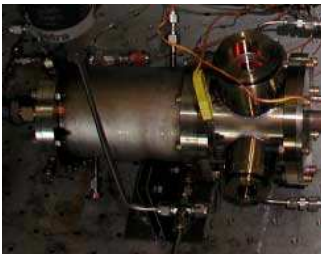
Figure 1. Partial oxidation reactor during operation with windows for carbon formation monitoring.
