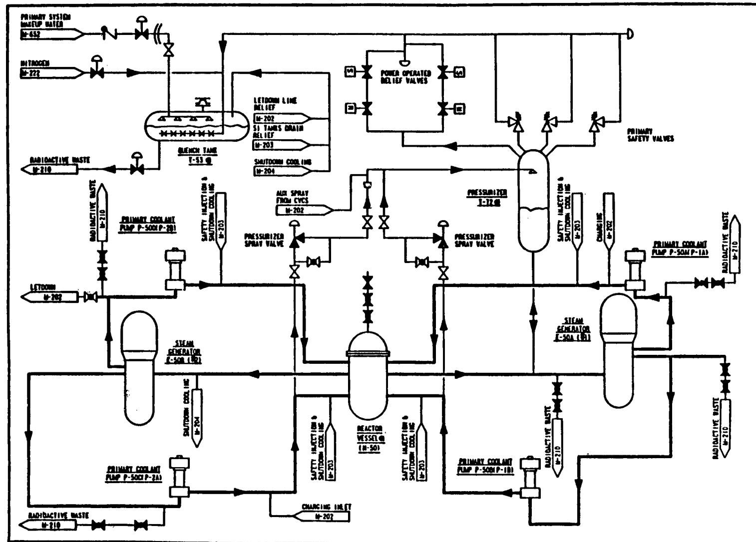
Figure 1.1 Primary coolant system flow
