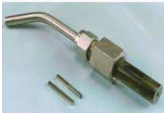
Figure 1. Potential application for the metallic-glass brazes joint. The MoSi 2 injector tube (bottom right of the figure) is joined to a stainless-steel adapter. The complexity of the joint makes the use of metallic-glass foils very attractive.
