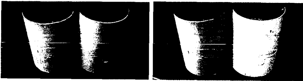
Figure 4-16. Overall views of the handrail specimen as it appeared as-received and after dividing in half (left), and after irradiation-aging of half of the specimen (right).
