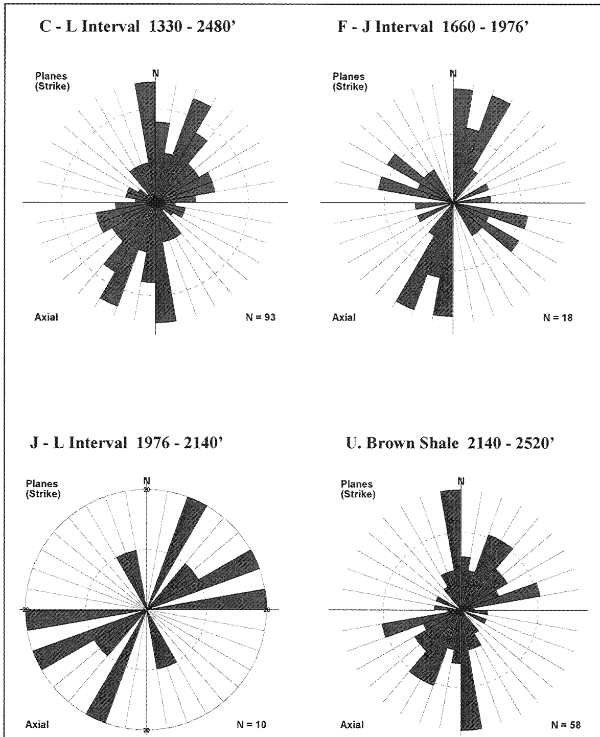
Figure 1.1-13. Azimuths of natural fractures as measured from the 12-8D EMI log. The CO 2 pilot will target the F-L interval. Note the increase in fractures and change in fracture azimuth in the Upper Brown Shale versus the F-J and J-L intervals. Data is from D. Julander and H. Wu.
