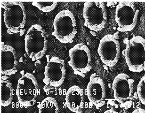
Figure 1.1-8. Opal-A frustule initiating conversion to opal-CT (left), and a frustule after its conversion to opal-CT. SEM photomicrographs, 10,000X magnification.
