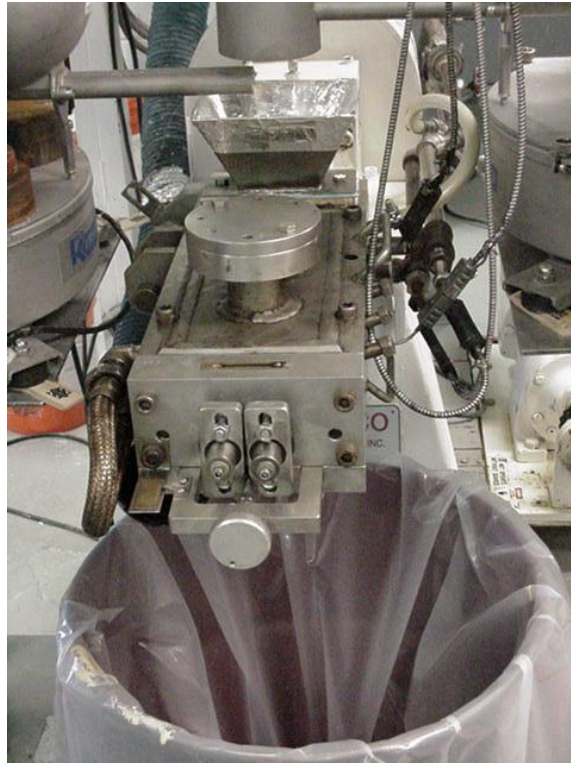
Figure 3. Readco Test Equipment Showing 2-Inch Mixer (Center) With Two Gravimetric Solid Feeders (Right and Left) And The Liquid Feed Pump (Lower Right).
