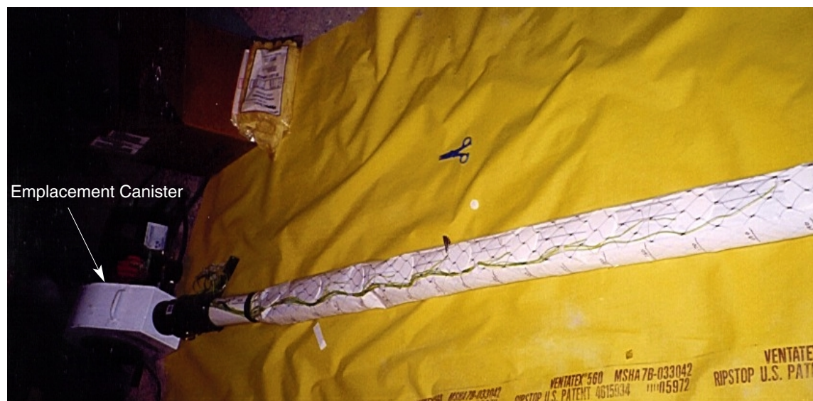
Figure 5. Emplacement Canister. The photo shows the pressurized emplacement canister and the collection membrane during initial installation of sampling pads.
