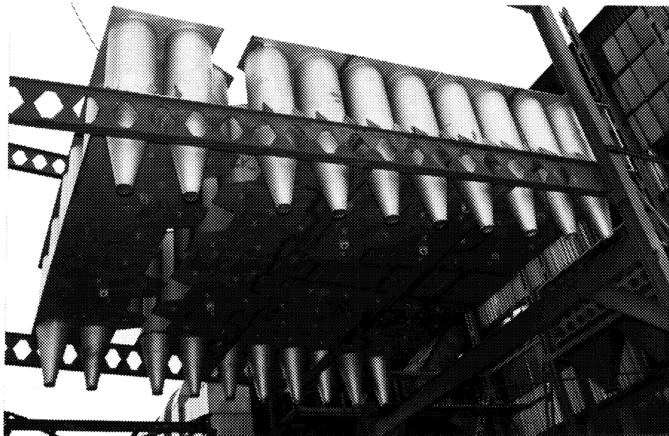
Figure 18. Core Separator Module Installation - FIAT AUTOPOLAND
