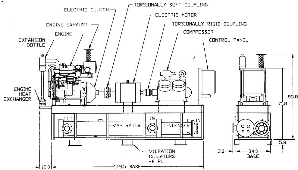
Alturdyne is searching for a consultant to perform a drive-line torsional analysis. This analysis is necessary to ensure that the drive-line is not subject to undue vibrations operating through its entire speed range.
