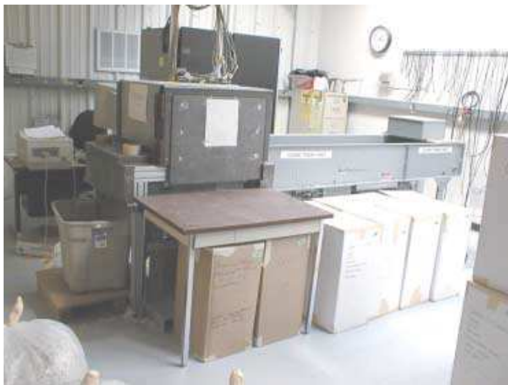
Figure 1. The WAND System. Detectors are housed to the left of the conveyor belt.
