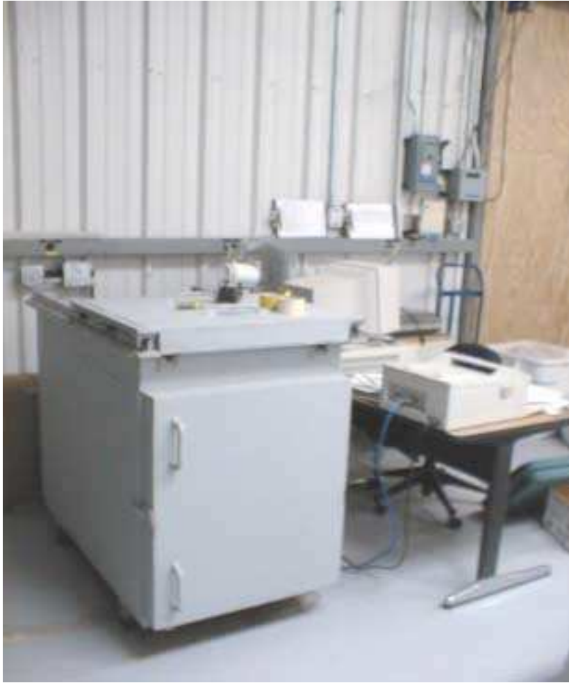
Figure 2. The HERCULES System. Detectors are housed on the near side of the chamber, waste is placed on the far side.
