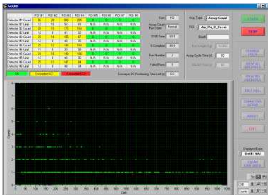
Figure 4. Detail of NaI spectrum from Detector #1 on a WAND system assay of a known plutonium source with an artificially long count.
