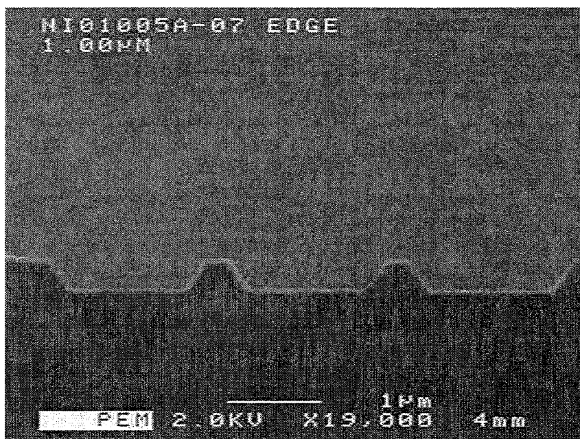
Figure 4. SEM of KOH-etched (100) silicon. The hard mask, which has been removed, was a filled space between an oxide line with an oxide spacer. The original 1.0 \mu\text{m} space was reduced to \sim 0.25 \mu\text{m} .
