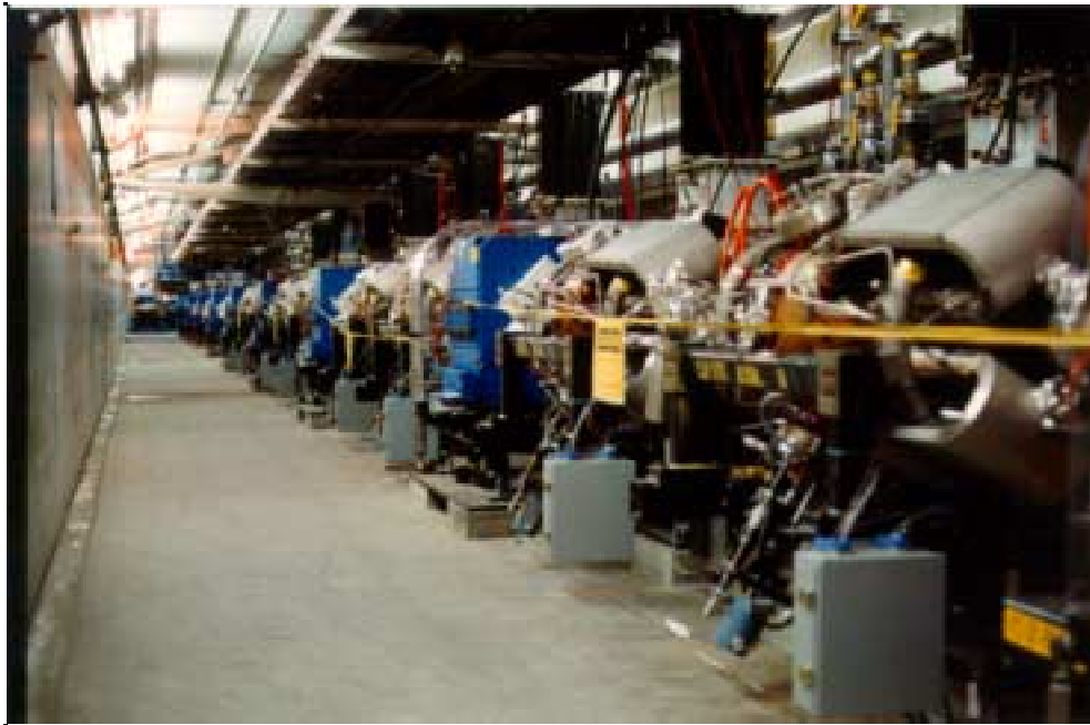
Figure 2: View of HER RF straight section. The curved waveguides on each cavity lead to damping loads that eliminate unwanted higher-order modes.
