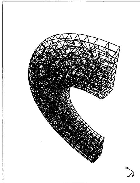
Figure 10: *Hexahedral Mesh on Half-Torus Geometry - After Untangle*
