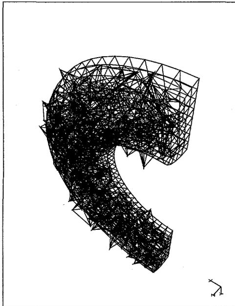
Figure 9: *Hexahedral Mesh on Half-Torus Geometry - Before Untangle*
