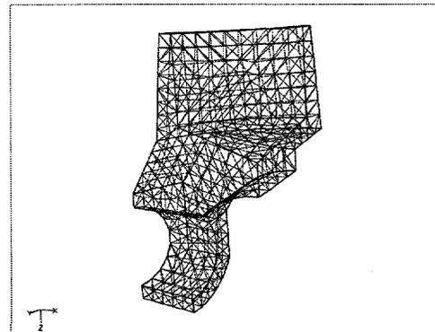
Figure 6: Tetrahedral Mesh on Hook Geometry
