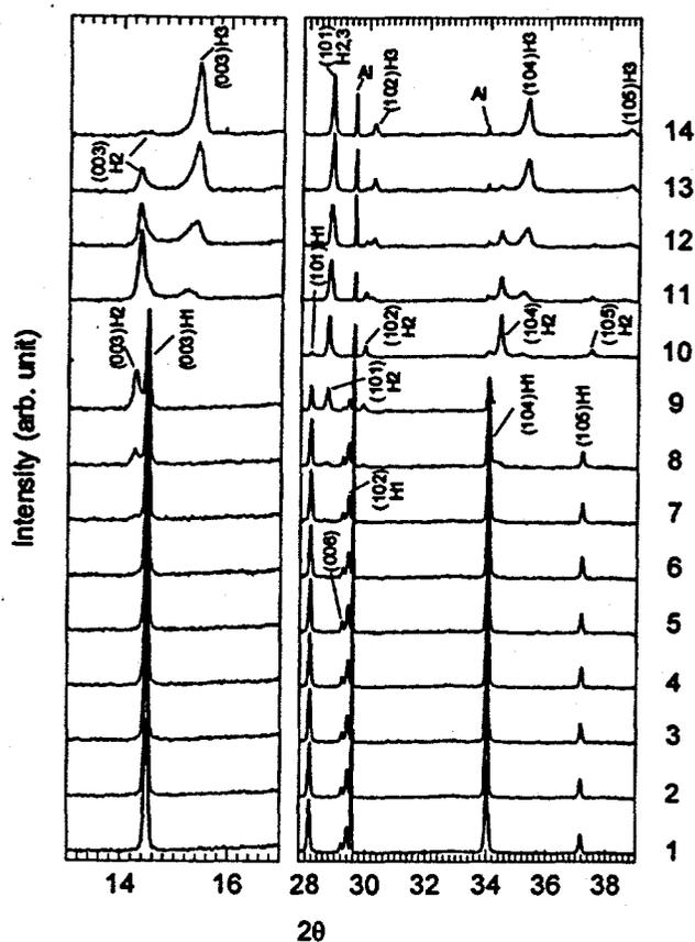
Figure 5 *In situ* XRD patterns for a  $\text{Li}_{1-x}\text{NiO}_2$  cathode in the (003) to (105) region of the hexagonal structure during first charge at the C/13 rate from 3.5 to 5.1 V, 66 min for each  $2\theta$  scan from  $13^\circ$  to  $54^\circ$  ( $\lambda=1.195 \text{ \AA}$ ).
