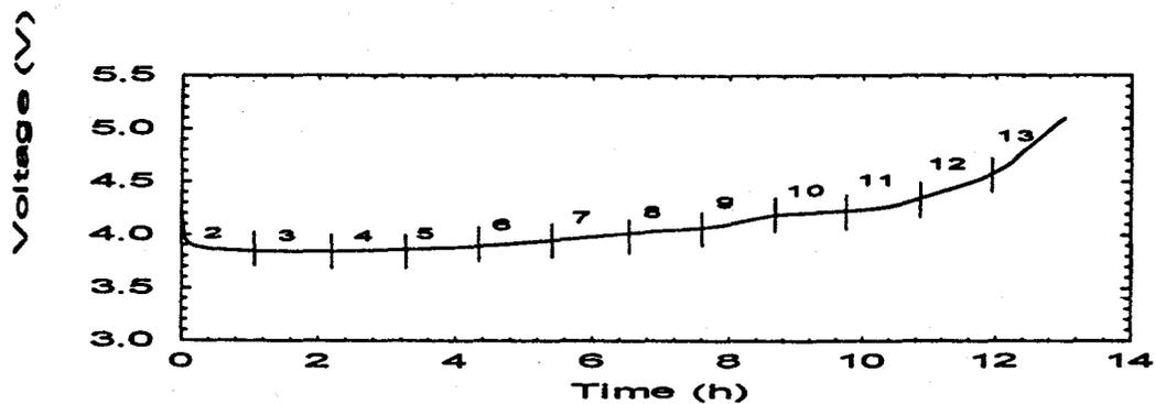
Figure 4. The first charging curve of a  $\text{Li}/\text{Li}_{1-x}\text{CNiO}_2$  cell at the C/13 rate from 3.5 to 5.1 V.
