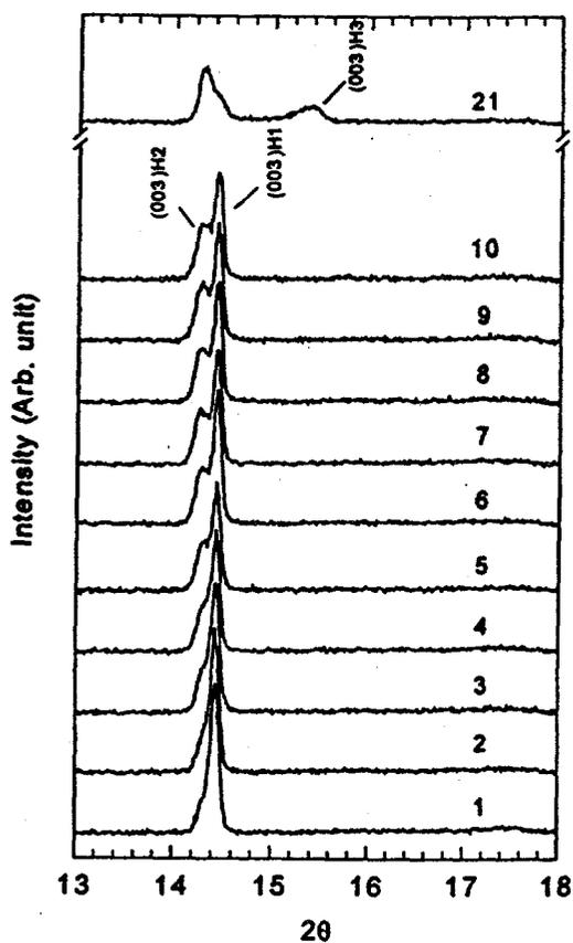
Figure 8 *In situ* XRD patterns for a  $\text{Li}_{1-x}\text{NiO}_2$  cathode in the (003) region of the hexagonal structure during first charge from 27 to 34.5 h and from 58.5 to 60.1 h (at the C/84 rate from 3.5 to 5.0 V) 1.65 h for each  $2\theta$  scan from  $13^\circ$  to  $54^\circ$  ( $\lambda=1.195 \text{ \AA}$ ).
