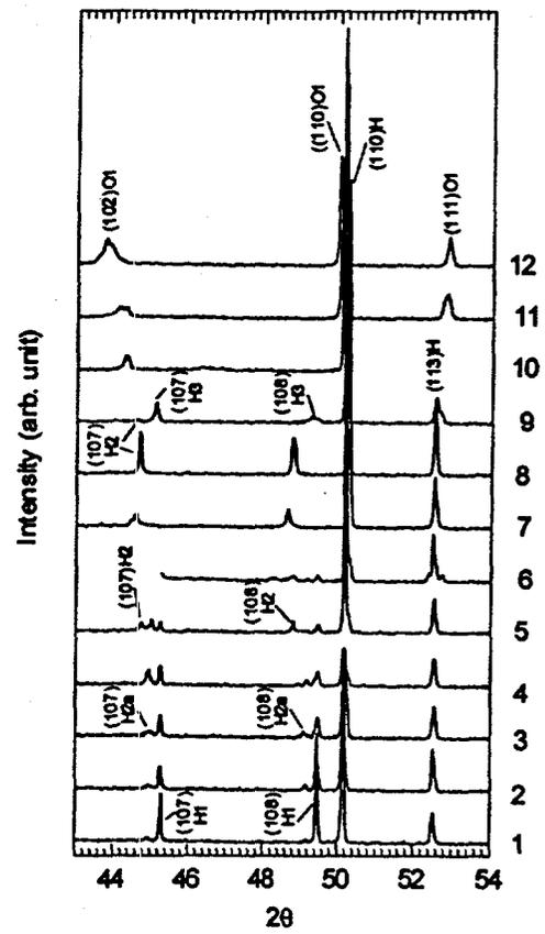
Figure 3 *In situ* XRD patterns for a  $\text{Li}_{1-x}\text{CoO}_2$  cathode in the (107) to (113) region of the hexagonal structure during first charge at the C/10 rate from 3.5 to 5.2 V, 50 min for each  $2\theta$  scan from  $13^\circ$  to  $54^\circ$  ( $\lambda=1.195 \text{ \AA}$ ).
