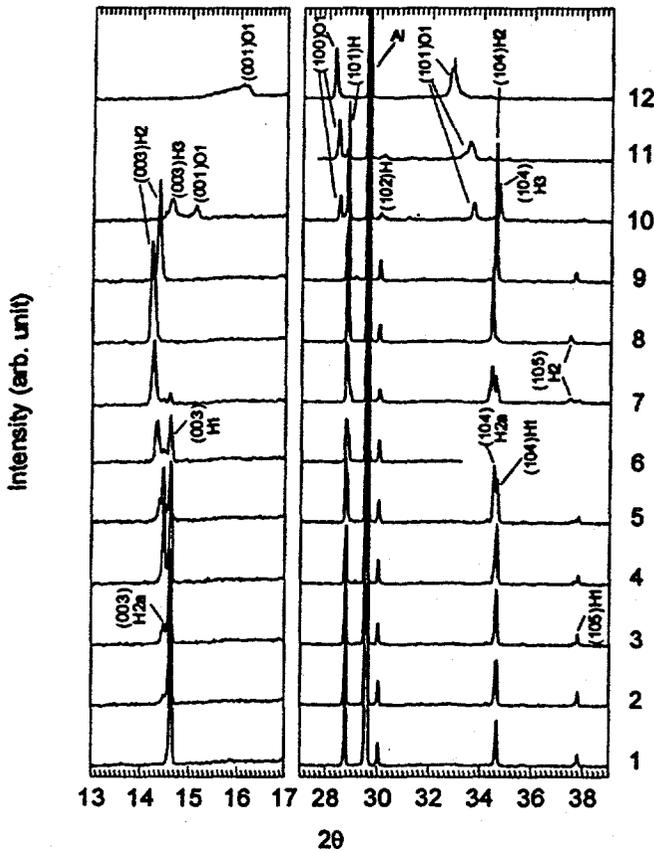
Figure 2 *In situ* XRD patterns for a  $\text{Li}_{1-x}\text{CoO}_2$  cathode in the (003) to (105) region of the hexagonal structure during first charge at the C/10 rate from 3.5 to 5.2 V, 50 min for each  $2\theta$  scan from  $13^\circ$  to  $54^\circ$  ( $\lambda=1.195 \text{ \AA}$ ).
