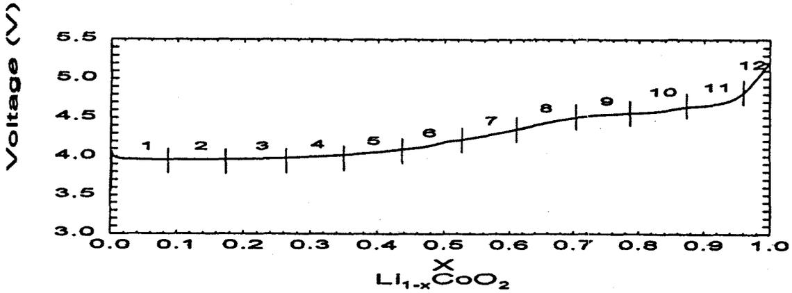
Figure 1. The first charging curve of a  $\text{Li}/\text{Li}_{1-x}\text{CoO}_2$  cell at the C/10 rate from 3.5 to 5.2 V.
