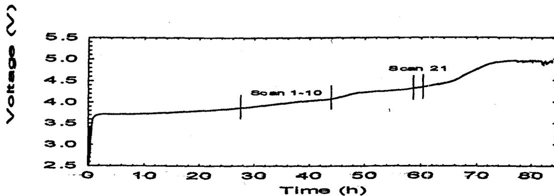
Figure 7. The first charging curve of a  $\text{Li}/\text{Li}_{1-x}\text{NiO}_2$  cell at the C/84 rate from 3.5 to 5.0 V.
