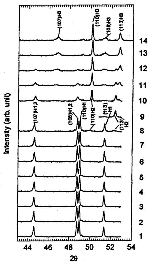
Figure 6 *In situ* XRD patterns for a  $\text{Li}_{1-x}\text{NiO}_2$  cathode in the (107) to (113) region of the hexagonal structure during first charge at the C/13 rate from 3.5 to 5.1 V, 66 min for each  $2\theta$  scan from  $13^\circ$  to  $54^\circ$  ( $\lambda=1.195 \text{ \AA}$ ).
