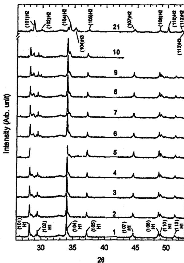
Figure 9 *In situ* XRD patterns for a  $\text{Li}_{1-x}\text{NiO}_2$  cathode in the (101) to (113) region of the hexagonal structure during first charge from 27 to 34.5 h and from 58.5 to 60.1 h (at the C/84 rate from 3.5 to 5.0 V) 1.65 h for each  $2\theta$  scan from  $13^\circ$  to  $54^\circ$  ( $\lambda=1.195 \text{ \AA}$ ).
