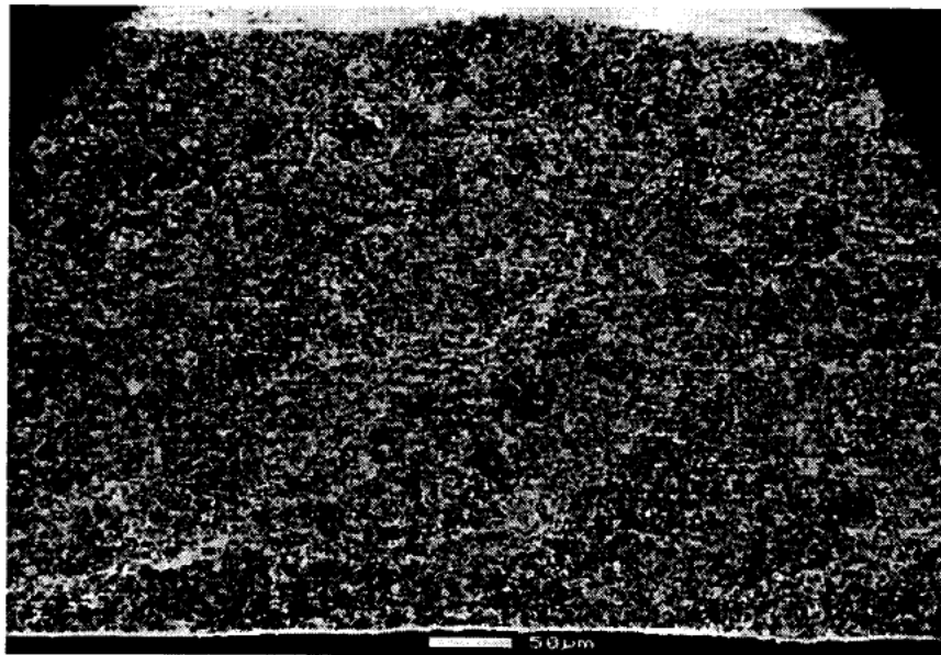
Fig. 47. Calendered Bilayer #B2B-B-4; sintered 1100°C/1h. Dense layer at bottom.
