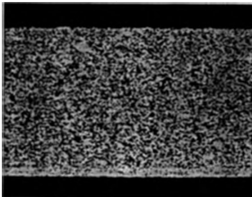
Figure 64. Calendered Bilayer #B2B-B-14; sintered 1050°C/1h. Dense layer at bottom. 250X
