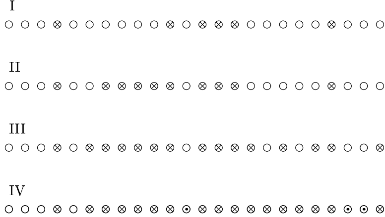
Figure 7. Snapshots of the failure process in a median strength ( N = 500 ) 2D HLLS \delta -bundle with 30 Weibull fibers and \rho = 1 under periodic boundary conditions. \circ intact fibers, \otimes broken fibers, and \odot first fibers to fail after instability.
