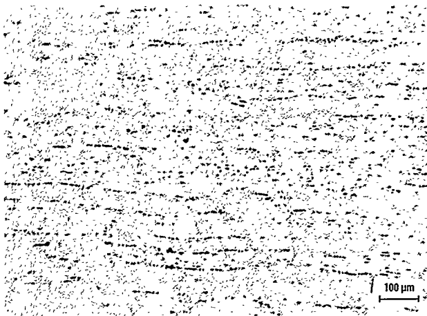
Figure 1 Microphotograph of annealed NiTi showing precipitant microstructures.
