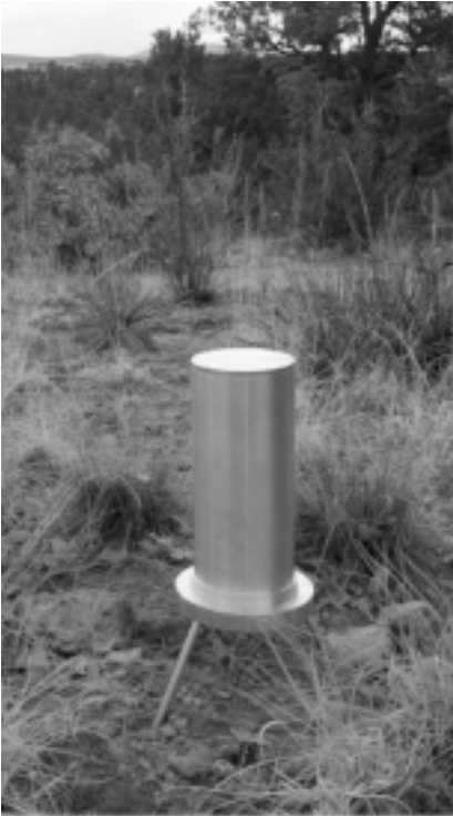
This compact, unattended infrasound sensor, developed at Los Alamos, has been used to demonstrate infrasound’s potential for facility characterization.
