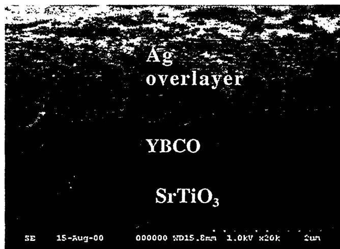
Fig. 5 Fracture surface of a YBCO film on an \text{SrTiO}_3 substrate. A columnar grain growth is evident, and the film appears to be dense.
