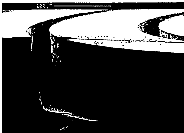
Fig. 6: SEM of a cross-section of a spiral GC column etched into Si using DRIE. The etch process results in deep, smooth, vertical channels.
