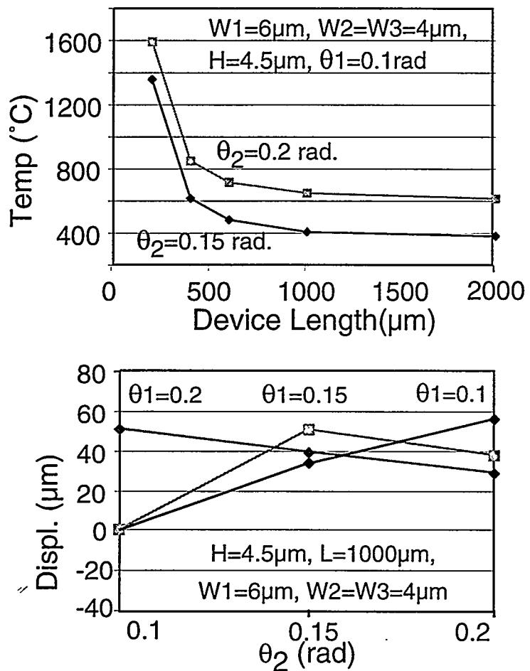
**Fig. 4:** FEA of orthogonal pairs, with 40  $\mu\text{N}$  external loading force, and non-linear expansion of Si. (a-upper) The maximum average operating temperature that can be achieved before out-of-plane buckling occurs; (b-lower) Lateral displacements that can be achieved before in-plane buckling occurs.
