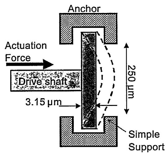
Fig. 6: Schematic of a loading beam used to measure output force available from an actuator.
