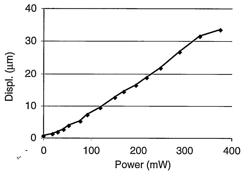
Fig. 10: Measured response of an isolated and unloaded Y-drive of the rotary actuator shown in Fig. 9. The maximum drive voltage used for this curve was 15 V.
