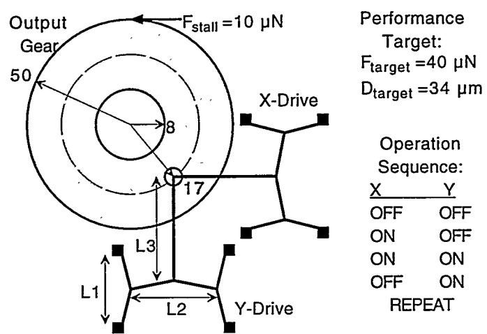
Fig. 2: Schematic (not to scale) of a rotary actuator based on orthogonal cascaded bent-beam elements for a gear of 50  $\mu\text{m}$  radius.
