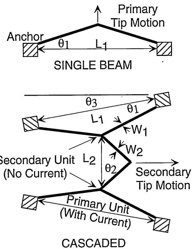
Fig. 1 The basic unit of the bent-beam thermal actuator (left), and a cascaded device (right).
