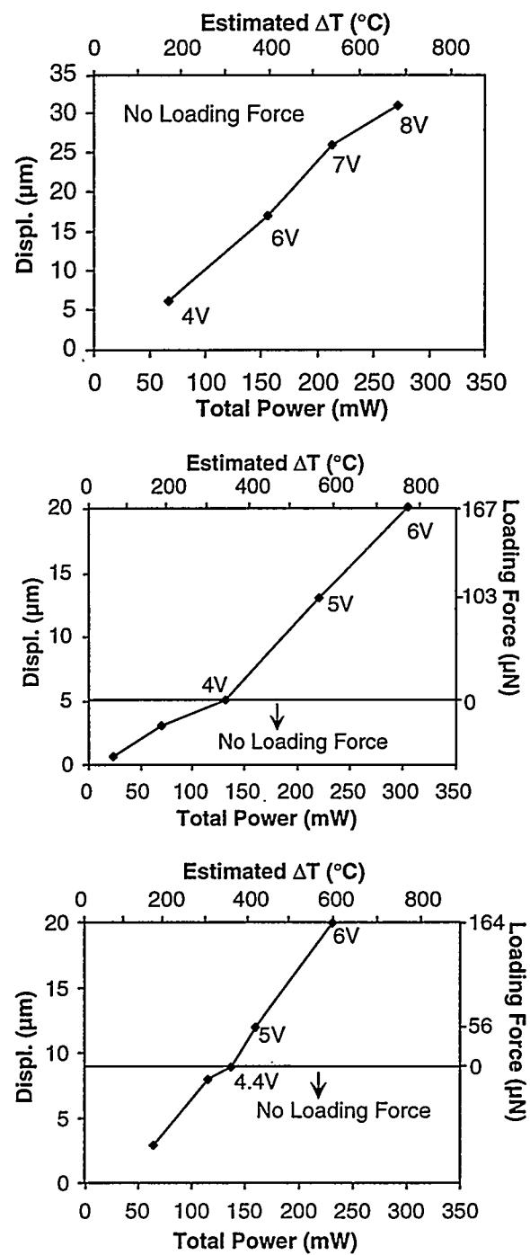
Fig. 7: (a: top-c: bottom) Displacement measurements of  $p^{++}$  Si rotary actuators R3, R5, and R6, respectively (Table I). In all cases the X and Y actuators were activated together.
