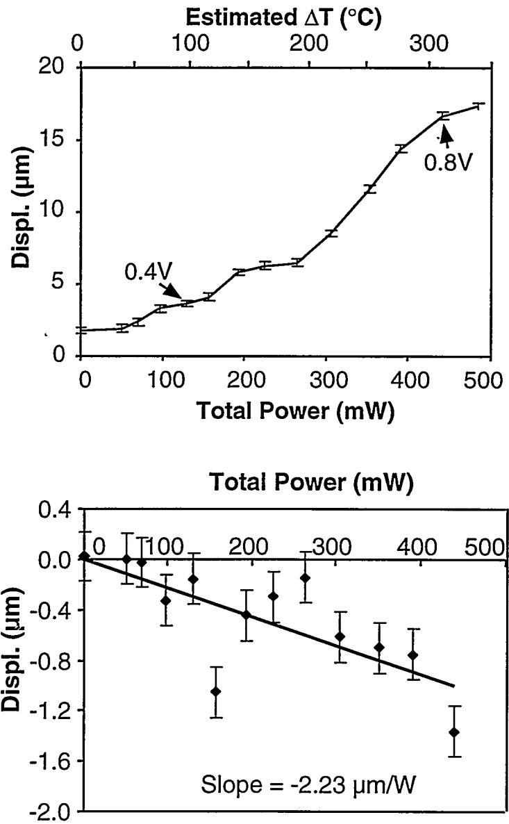
Fig. 8: Measured results of electroplated Ni rotary actuator RJ3 (Table I) with only one axis actuated: (a-upper) the forward displacement of the actuated axis; and (b-lower) a small backward displacement along the orthogonal axis which can be easily compensated.
