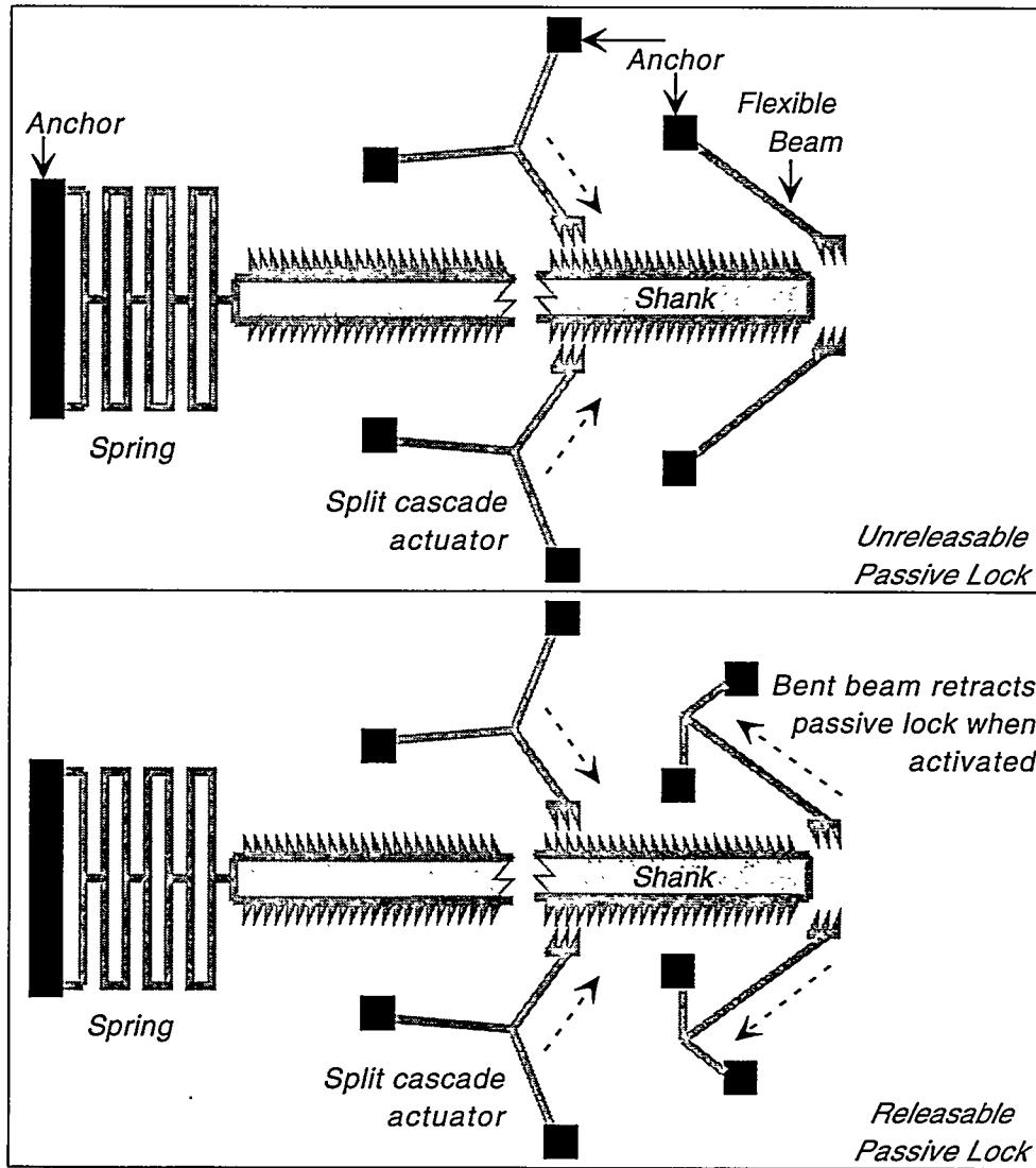
Fig. 12: (a-upper) An inchworm actuator with passive lock that will prevent the pull-back of the shank when power to the actuator is turned off; (b-lower) An inchworm with a retractable passive lock.
