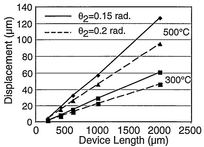
**Fig. 3:** Non-linear FEA of an orthogonal pair of cascaded Si actuators with one axis actuated. Dimensions:  $W_1=6 \mu\text{m}$ ,  $W_2=W_3=4 \mu\text{m}$ ,  $\theta_1=0.1\text{rad.}$ ,  $H=4.5 \mu\text{m}$ , and  $L_1=L_2=L_3$ .
