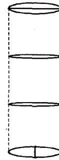
Figure 12. Three stacked cylinders that are individually many-to-one or one-to-one sweepable. The collection taken together is only meshable with MultiSweeping.
