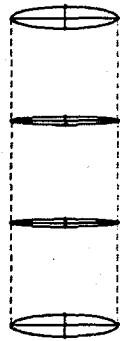
Figure 14. Three stacked cylinders after the source surfaces have been imprinted with the target surface topology.
