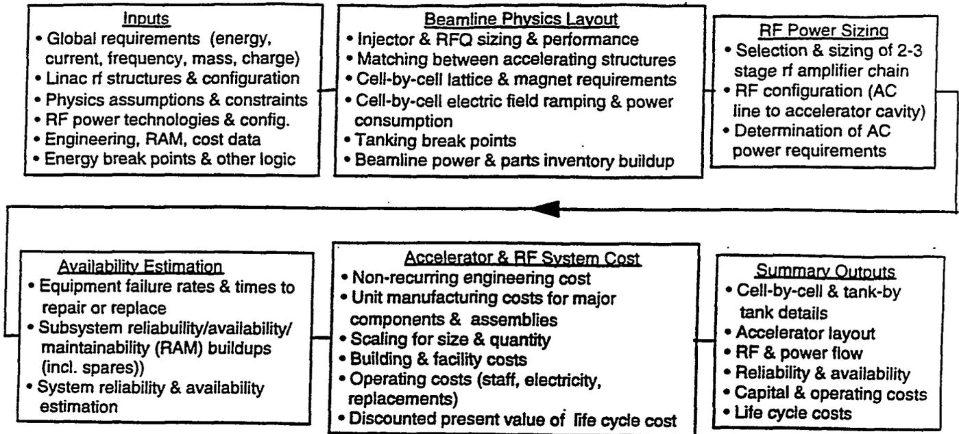
As shown in Fig. 1, the first series of Fortran routines use the input data to establish a cell-by-cell layout of the accelerator, starting at the ion injector and proceeding through all of the major rf structures, completing each at a specified energy breakpoint. A generalized set of algorithms is used to match the synchronous phase and the longitudinal and transverse phase advances from structure to structure.
